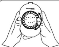
Rotate the main button counter clockwise (past 00:00) to delete the setting. The remaining time periods will be rearranged in order.
