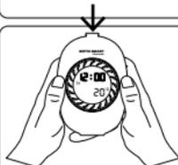
Press the main button to enter the Time setting stage. The time will be flashing.
