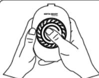
Press and hold the main button for 3 sec. to complete the setting.
