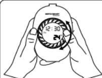
Rotate the main button clockwise or counter clockwise to increase or decrease the temperature. (20°C to 50°C).
